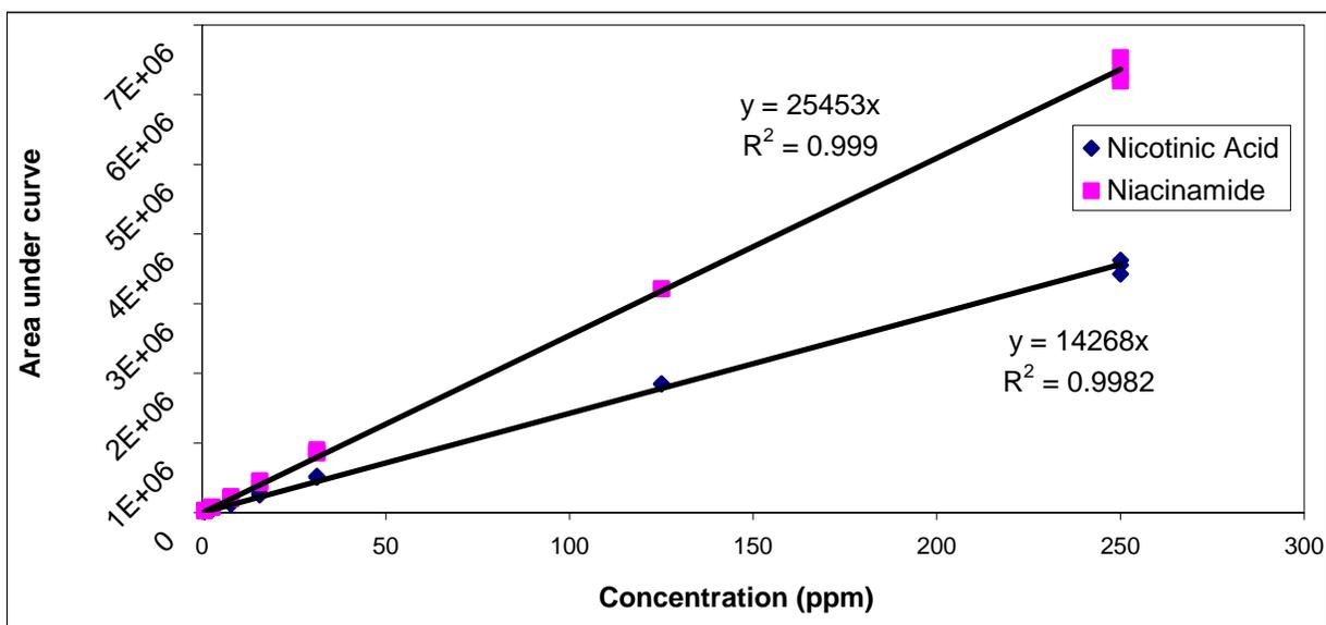
Figure 3. Calibration curve of nicotinic acid and niacinamide with a concentration range from 3ppm to 250 ppm. Linear regression lines and R2 values are displayed on the graph.
