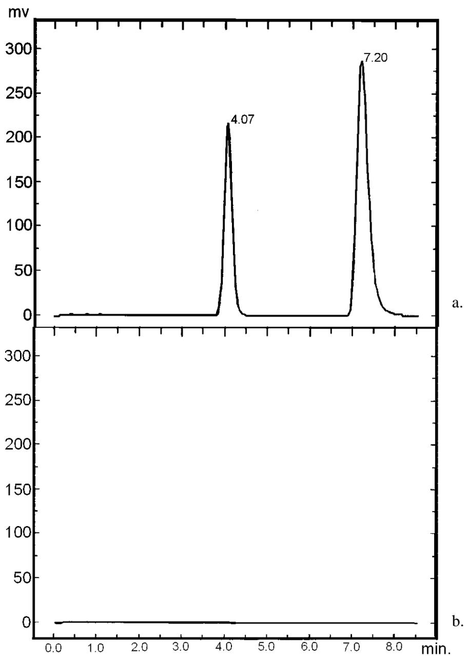
Figure 2. a. Chromatogram of nicotinic acid, eluting at 4.07 min and niacinamide, eluting at 7.20min. with photolysis unit on. b. chromatogram of nicotinic acid and niacinamide with photolysis unit off.
